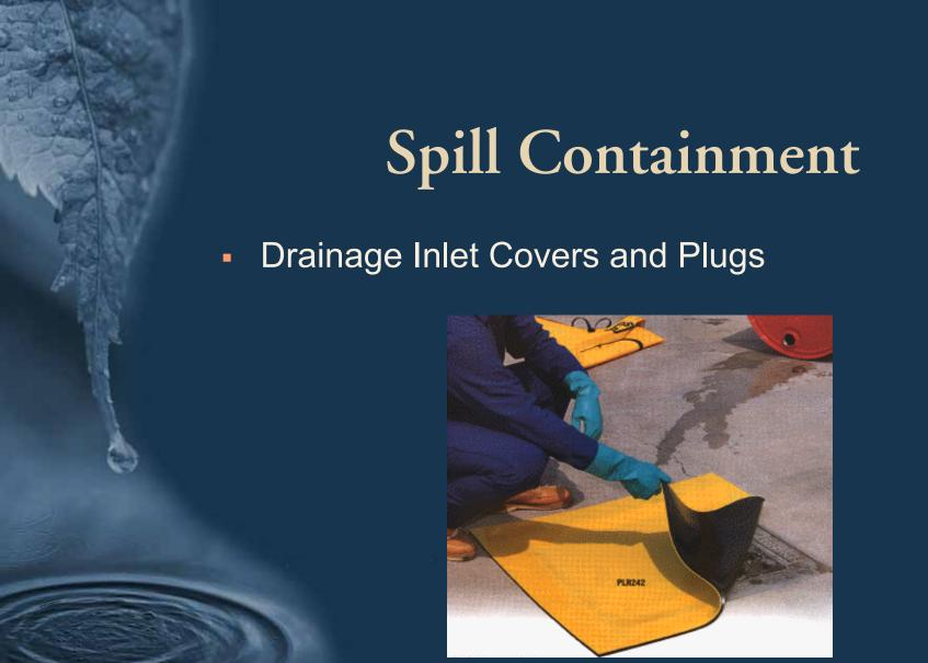
Drainage inlet cover (Photo courtesy of New Pig Corporation)
